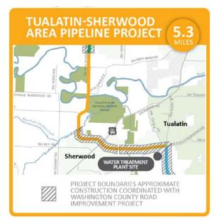
The Tualatin-Sherwood Area Pipeline Project is a 5.3-mile section of the 30-mile Willamette Water Supply System pipeline, about half of which is a partnership with Washington County. This section of the pipeline, a 66-inch welded steel pipe with a cement lining, will be constructed in coordination with the <u>Washington County Major Streets Transportation Improvement Program</u> projects on Tualatin Sherwood Road.
